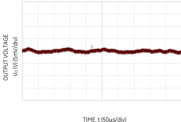
Figure 15. Typical output ripple and noise ( $C_O=12 \times 47\mu F$  ceramic +  $10 \times 470\mu F$  polymer,  $V_{IN} = 12V$ ,  $I_o = I_{o,max.}$ )
