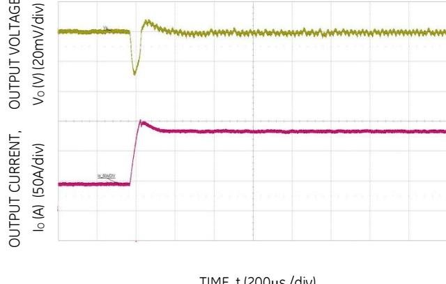
Figure 22. Transient Response to Dynamic Load Change from 25% to 75% at 12Vin,  $C_o = 12 \times 47\mu F + 10 \times 1000\mu F$ ,  $R_{TUNE} = 3.01k\Omega$ .
