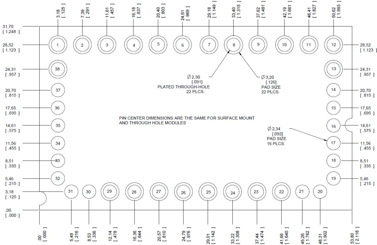
Note: In the Through-Hole version of the TJT170, pins 1-13, 22-29 and 38 are Through-Hole pins, pins 14-21, 30-37 are SMT pins. The drawing above shows the recommended layout as a combination of holes in the PWB to accommodate the Through-Hole pins and pads on the top layer to accommodate the SMT pins.
