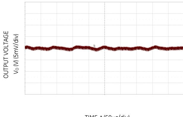
Figure 9. Typical output ripple and noise ( $C_o = 12 \times 47\mu F$  ceramic +  $10 \times 470\mu F$  polymer,  $V_{IN} = 12V$ ,  $I_o = I_{o,max}$ )
