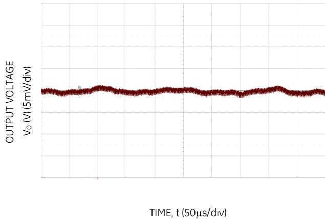
Figure 3. Typical output ripple and noise ( $C_o = 12 \times 47\mu F$  ceramic +  $10 \times 470\mu F$  polymer,  $V_{IN} = 12V$ ,  $I_o = I_{o,max}$ ).
