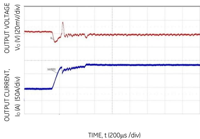
Figure 4. Transient Response to Dynamic Load Change from 25% to 75% at 12Vin,  $C_o = 12 \times 47\mu F + 10 \times 1000\mu F$ ,  $R_{TUNE} = 3.01k\Omega$ .
