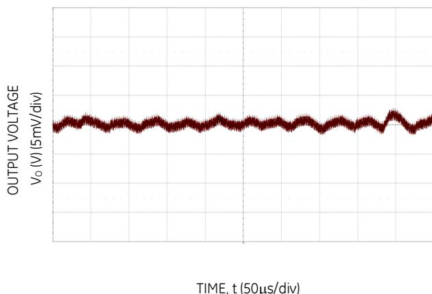
Figure 27. Typical output ripple and noise ( $C_o=12 \times 47\mu F$  ceramic +  $10 \times 470\mu F$  polymer,  $V_{IN} = 12V$ ,  $I_o = I_{o,max}$ )
