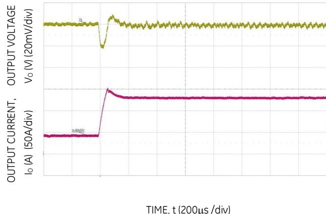
Figure 16. Transient Response to Dynamic Load Change from 25% to 75% at 12Vin,  $C_O = 12 \times 47\mu F + 10 \times 1000\mu F$ ,  $R_{TUNE} = 3.01k\Omega$ .
