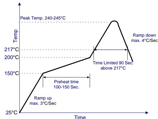
Figure 39. Recommended linear reflow profile using Sn/Ag/Cu solder.
