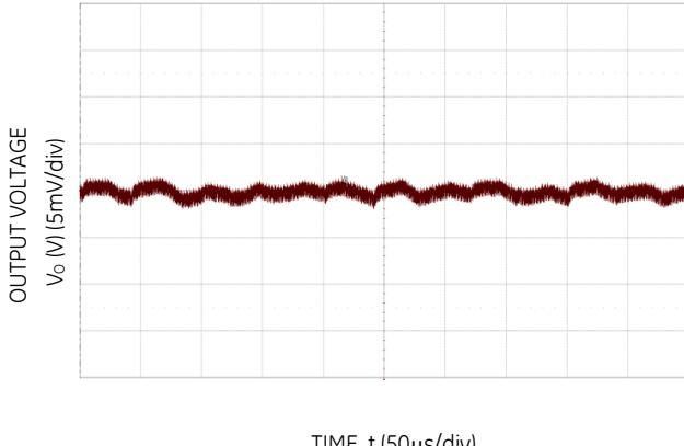
Figure 21. Typical output ripple and noise ( $C_o = 12 \times 47\mu F$  ceramic +  $10 \times 470\mu F$  polymer,  $V_{IN} = 12V$ ,  $I_o = I_{o,max}$ )
