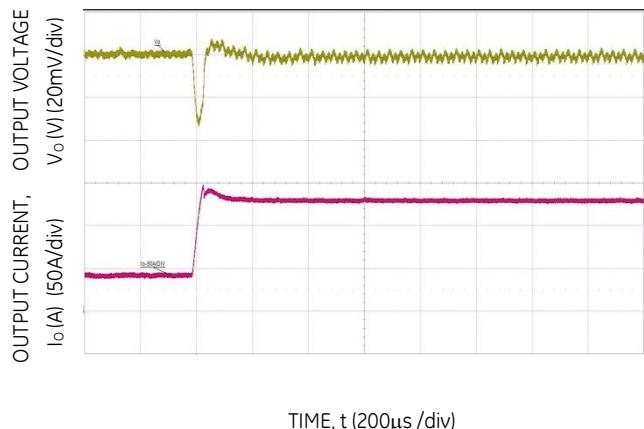
Figure 28. Transient Response to Dynamic Load Change from 25% to 75% at 12Vin,  $C_o= 12 \times 47\mu F + 10 \times 1000\mu F$ ,  $R_{TUNE} = 3.01k\Omega$ .
