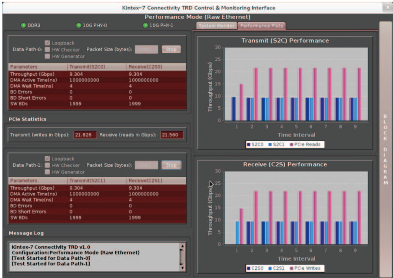
Figure 2-24: Raw Ethernet Driver Performance Plots
