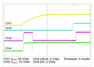
Figure 14 — Start up from application of V<sub>PRI\_DC</sub>= 42 V, 20% I<sub>OUT</sub>, 100% C<sub>SEC\_OUT\_EXT</sub>
