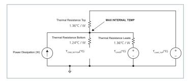
Figure 20 — Top case and leads thermal model
