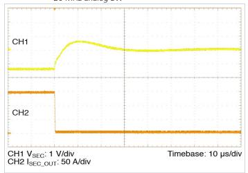
**Figure 13** — 160 A – 0 A transient response:  $C_{IN} = 270 \, \mu F$ , no external  $C_{SFC\ OUT\ FXT}$
