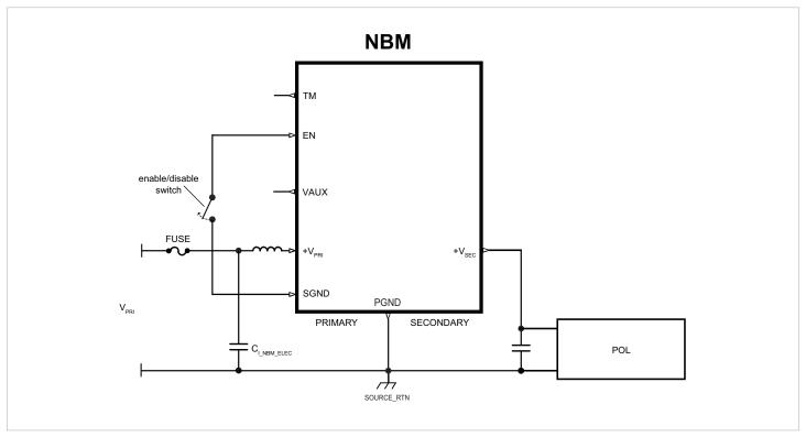
NBM6123x46C15A6yzz+ Point of Load
