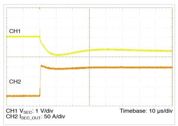
**Figure 12** — 0 A– 160 A transient response:  $C_{PRI\ OUT\ EXT} = 270\ \mu\text{F}$ , no external  $C_{SEC\ OUT\ EXT}$
