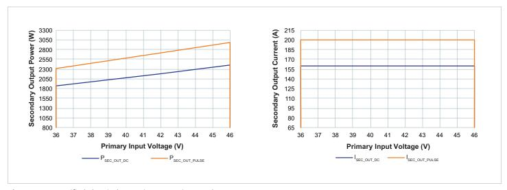
**Figure 2** — Specified electrical operating area using rated R<sub>SEC\_HOT</sub>
