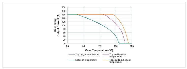
Figure 1 — Specified thermal operating area
