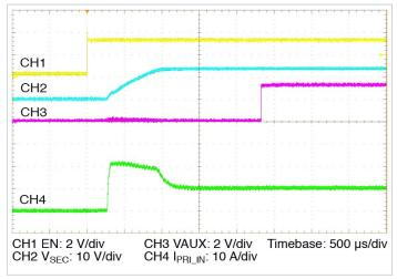
**Figure 15** — Start up from application of EN with pre-applied  $V_{PRI\_DC} = 42 \text{ V}$ , 20%  $I_{SEC\_DG}$ , 100%  $C_{SEC\_OUT\_EXT}$
