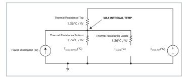
Figure 21 — Top case thermal model
