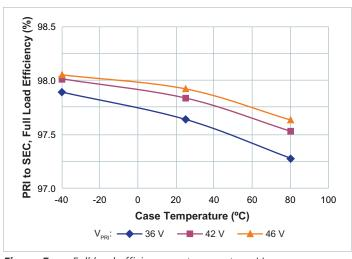
**Figure 5** — Full load efficiency vs. temperature; V<sub>PRI\_DC</sub>
