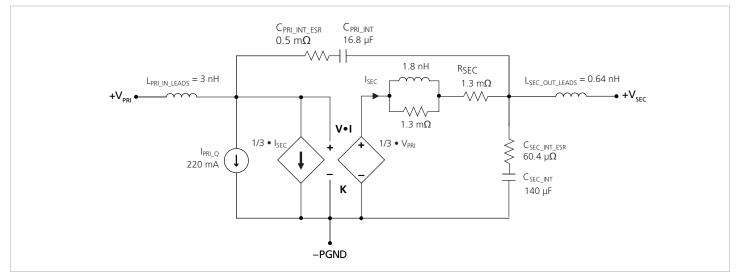
Figure 16 — NBM module AC model
