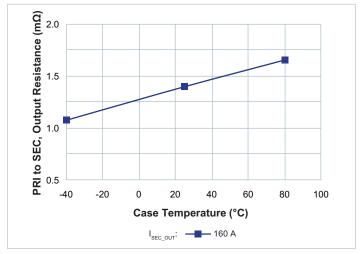
Figure 9 —  $R_{OUT}$  vs. temperature; Nominal  $V_{PRI\_DC}$  $I_{SEC\_DC} = 160$  A at  $T_{CASE} = 80$ °C
