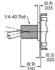
When using this bushing, toggle length is increased by .070" (1.78mm). Maximum Panel Thickness with Standard Hardware: .031" (0.8mm)
