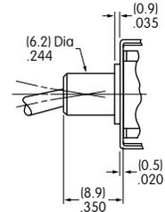
When using this bushing, toggle length is increased by .070" (1.78mm).
