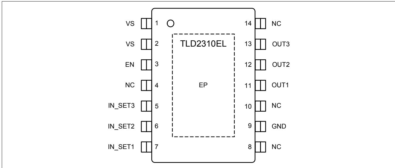
Figure 2 Pin Configuration
