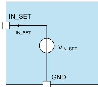
**Figure 7** Block Diagram IN\_SET pin
