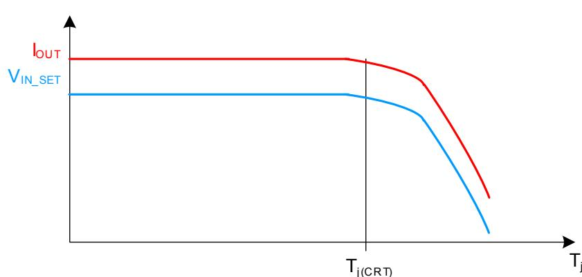
**Figure 11 Output current reduction at high temperature**
