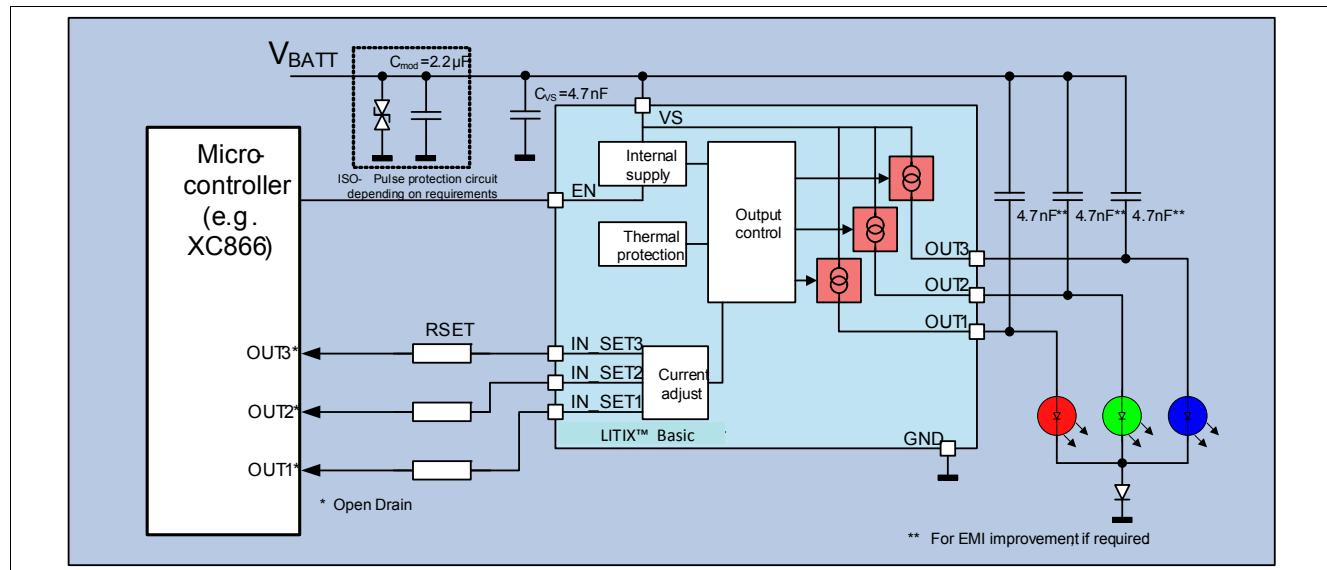
**Figure 12 Application Diagram**
