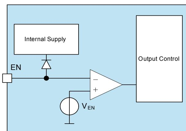
**Figure 3 Block Diagram EN pin**
