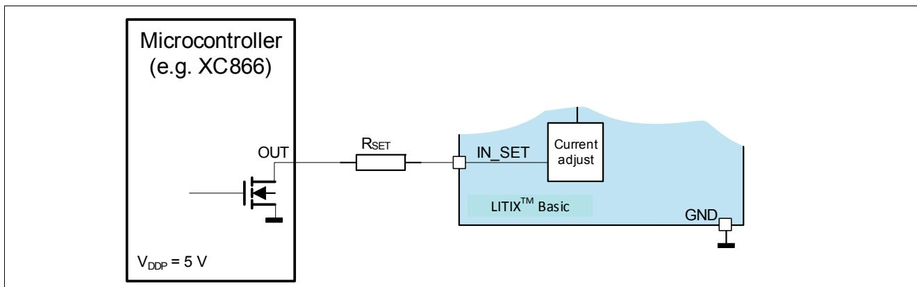
**Figure 8** Schematics IN\_SET interface to µC
