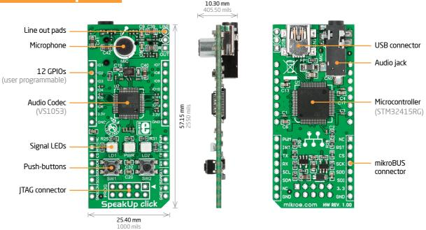
Along with its key components, the SpeakUp packs other useful bits like two buttons for recording or deleting voice commands manually, while three signal LEDs give recognition feedback and indicate power.
