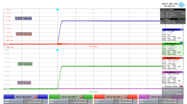
Figure 37 – Output Voltage and Current Waveforms. 265 VAC Input. Upper: 12 V, 2 V / div. Lower: 5 V, 1 V, 10 ms / div.
