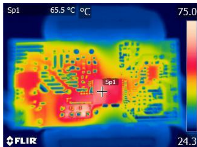
Figure 19 – InnoSwitch3-EP Side. 90 VAC, Full Load.
