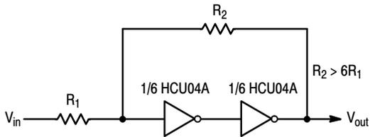
Figure 6. Schmitt Trigger
