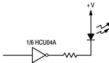
For reduced power supply current, use high-efficiency LEDs such as the Hewlett-Packard HLMP series or equivalent.
