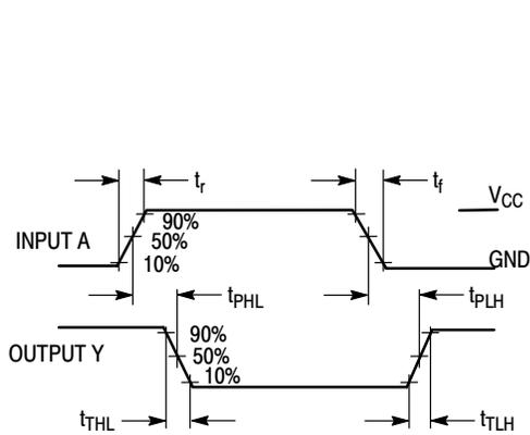
Figure 1. Switching Waveforms
