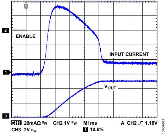
Figure 26. Typical Turn-On Time and Inrush Current,  $V_{IN} = 5$  V,  $C_{OUT} = 47 \mu\text{F}$ ,  $330 \Omega$  Load
