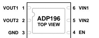
Figure 4. 6-Lead LFCSP Pin Configuration
