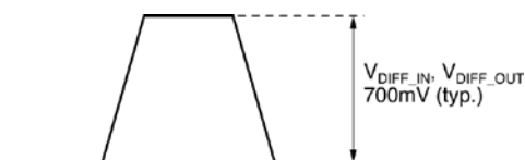
Figure 1b. Differential Voltage Swing
