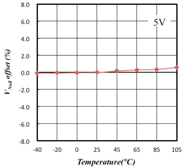
Figure 2. Output Voltage Offset vs. Temperature
