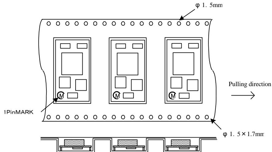
The module is located such as inductor in upper side and terminal in lower side.
