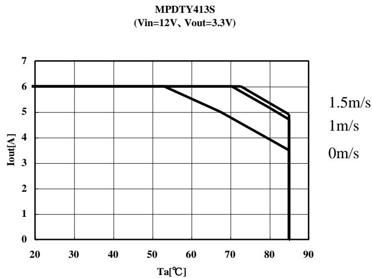
When using this product at the ambient air temperature of 55°C more, it is used by the following temperature derating.
