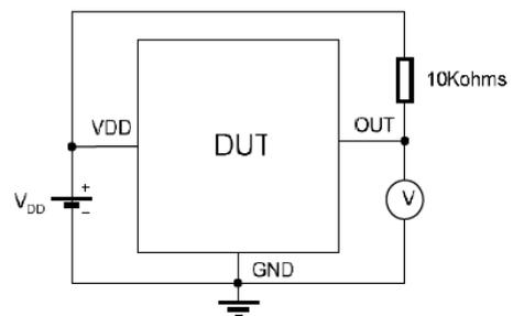
Note 1 -  $B_{Op}$  is determined by putting the device under magnetic field swept from  $E_{RPmin}$  up to  $B_{OPmax}$  until the output is switched on.
