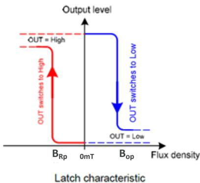
Typically, the device behaves as a latch with symmetric operating and release switching points ( $B_{Op} = |B_{Rp}|$ ). This means magnetic fields with equivalent strength and opposite direction drive the output high and low.
