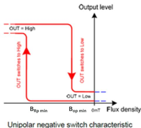
In latch, positive or negative switch behaviour, a magnetic hysteresis  $B_{Hyst}$  keeps  $B_{Op}$  and  $B_{Rp}$  separated by a minimal value. This hysteresis prevents output oscillation near the switching point.
