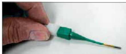
Plastic tool with contact in proper position.
