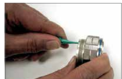
Plastic tool with contact in proper position.
