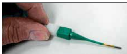
Plastic tool with contact in proper position.
