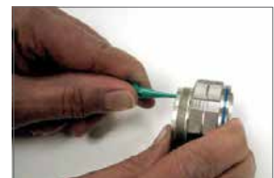
Plastic tool with contact in proper position.
