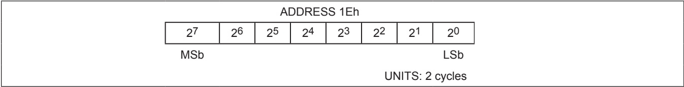
Figure 12. Cycle Counter Register Format
