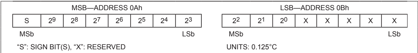
Figure 5. Temperature Register Format
