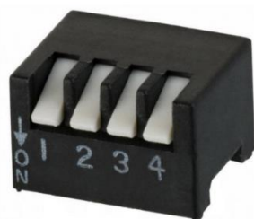
Figure 7.2. Four-Position DIP Switch Photograph
