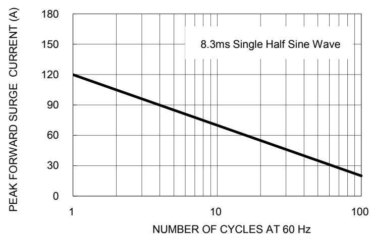
FIG. 2 MAXIMUM NON-REPETITIVE FORWARD SURGE CURRENT PER LEG
