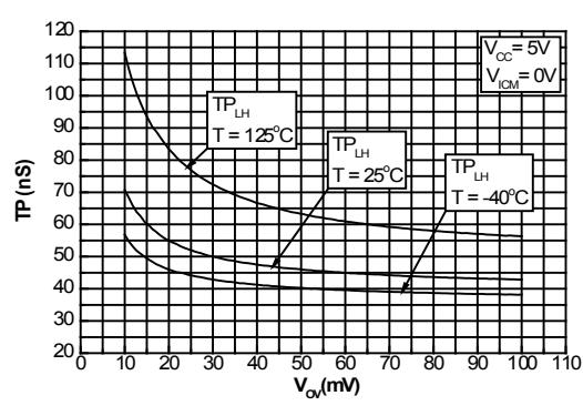
**Figure 25. Propagation delay (LH) vs. overdrive at  $V_{CC} = 5\text{ V}$ ,  $V_{ICM} = V_{CC}$**
