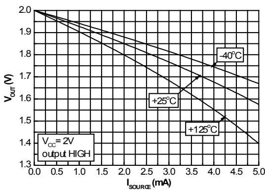
**Figure 6. Output voltage vs. sink current, V<sub>CC</sub> = 2 V**
