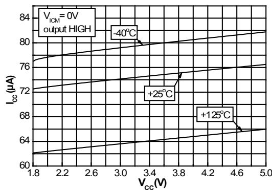
**Figure 2. Current consumption vs. supply voltage (V<sub>ICM</sub> = V<sub>CC</sub>, output high)**
