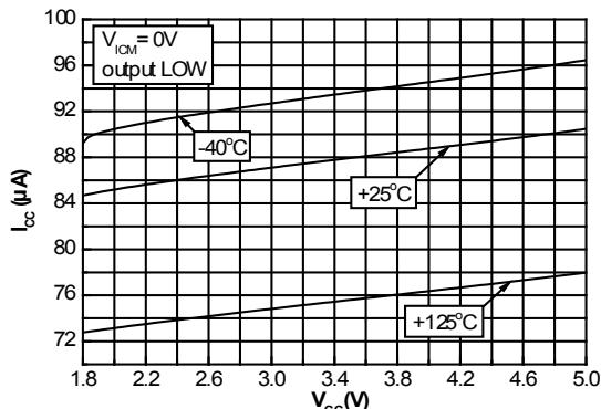
**Figure 4. Current consumption vs. supply voltage (V<sub>ICM</sub> = V<sub>CC</sub>, output low)**
