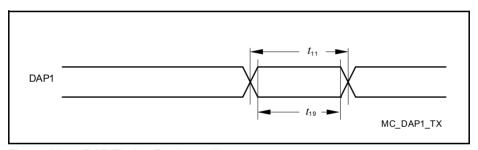
Figure 29 DAP Timing Device to Host
