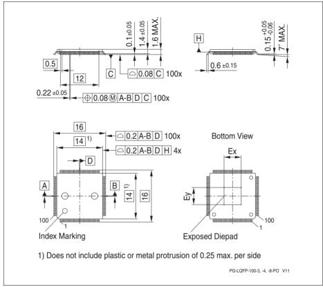
Figure 32 PG-LQFP-100-8/-15 (Plastic Green Thin Quad Flat Package)
