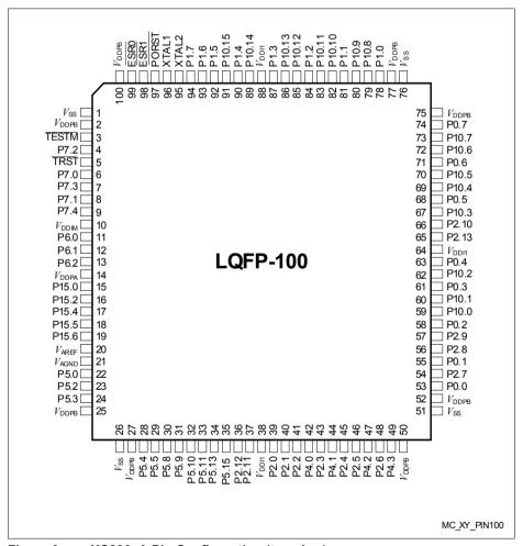
Figure 3 XC236xA Pin Configuration (top view)
