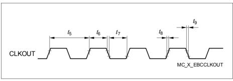
Figure 22 CLKOUT Signal Timing
