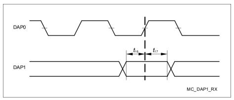
Figure 28 DAP Timing Host to Device
