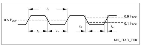
Figure 30 Test Clock Timing (TCK)
