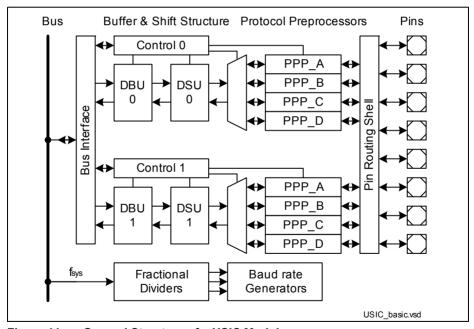
Figure 11 General Structure of a USIC Module
