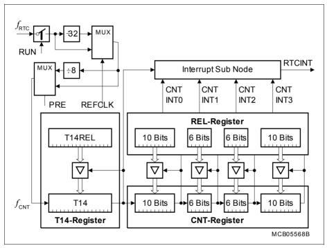
Figure 10 RTC Block Diagram
