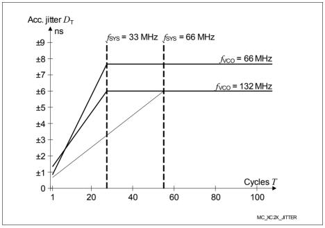
Figure 20 Approximated Accumulated PLL Jitter
