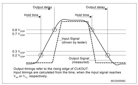
Figure 17 Input Output Waveforms
