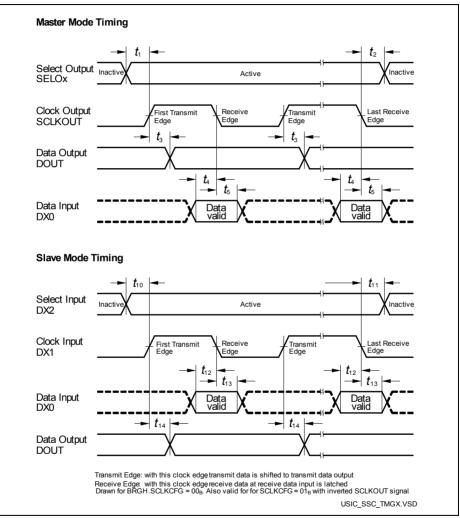
Figure 26 USIC - SSC Master/Slave Mode Timing
