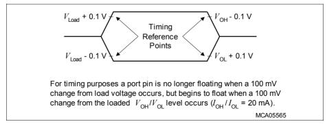
Figure 18 Floating Waveforms
