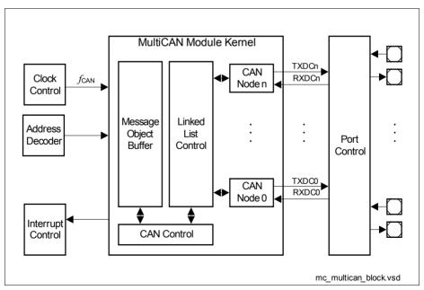
Figure 12 Block Diagram of MultiCAN Module
