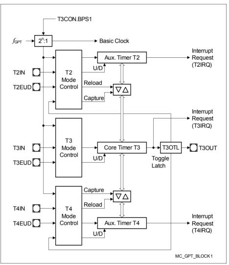
Figure 8 Block Diagram of GPT1
