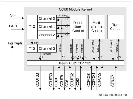
Figure 7 CCU6 Block Diagram
