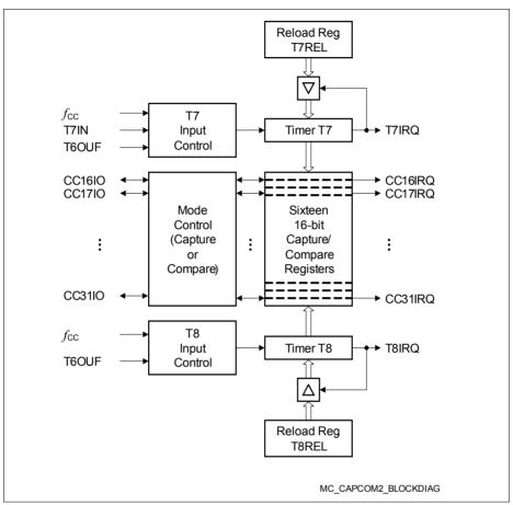
Figure 6 CAPCOM2 Unit Block Diagram
