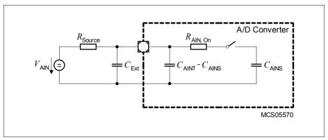
Figure 16 Equivalent Circuitry for Analog Inputs
