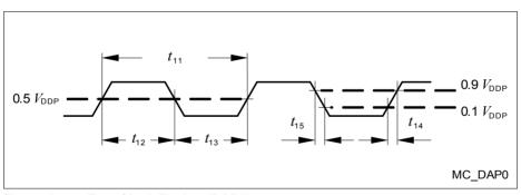
Figure 27 Test Clock Timing (DAP0)
