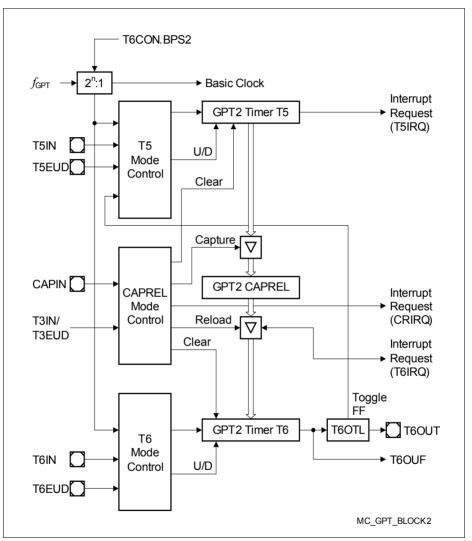
Figure 9 Block Diagram of GPT2
