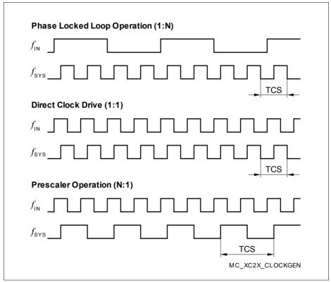
Figure 19 Generation Mechanisms for the System Clock
