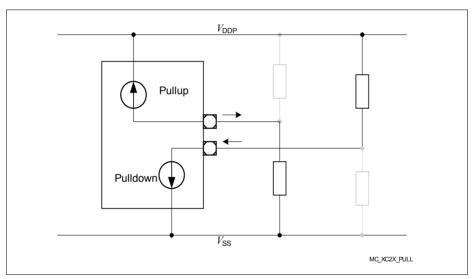
Figure 13 Pullup/Pulldown Current Definition
