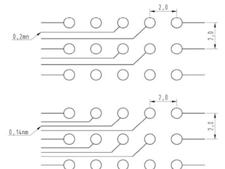
Under the condition that the width of the track and the space between should be equal, two tracks of 0.2mm width or three tracks of 0.14mm width can be placed between two rings.
