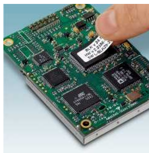
Stick-on device marking, removable, for printing with THERMOMARK ROLL... EML-RM... Page 277
