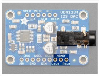
The exciting part! This is where your line level audio comes out. We put big 47uF blocking capacitors on the output so you can connect this to any stereo system.
