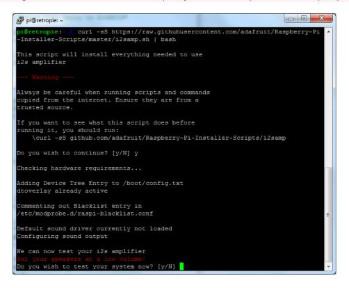
We've added an extra helper systemd script that will play quiet audio when the I2S peripheral isn't in use. This removes popping when playback starts or stops. It uses a tiny amount of CPU time (on a Pi Zero, 5%, on a Pi 2 or 3 its negligible). You don't need this on RetroPie because it never releases the I2S device, but it's great for Raspbian.
