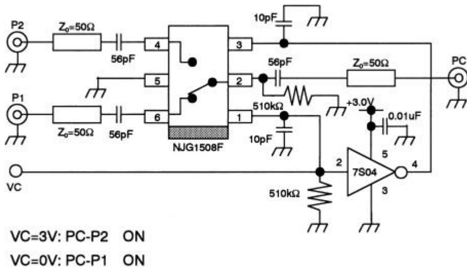
[1]Please connect bypass capacitors to the supply terminals of the C-MOS inverter.
