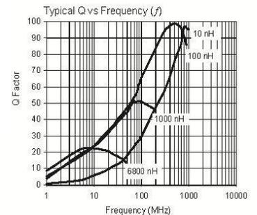
**Features:** Gold pad metallization, For surface mount assembly, High Q
