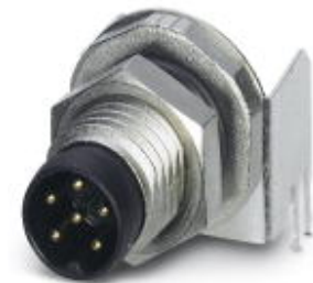
Sensor/actuator flush-type plug-in connector, plug, 6-pos., M8, rear/screw mounting with M8 fastening thread, with angled solder connection
