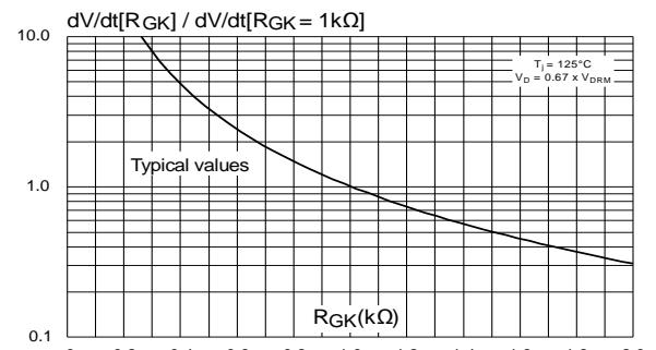
**Figure 7: Relative variation of dV/dt immunity versus gate-cathode capacitance**
