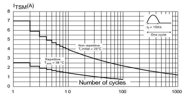
**Figure 9: Non-repetitive surge peak on-state current for sinusoidal pulse ( $t_p < 10$  ms)**
