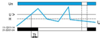
Tt Time delay after crossing of threshold (adjustable on front panel from 0.3 s to 30 s)
