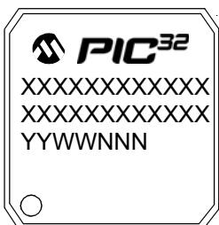
100-Lead TQFP (12x12x1 mm)
