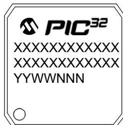
100-Lead TQFP (14x14x1 mm)
