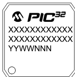
100-Lead TQFP (12x12x1 mm)
