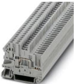
Feed-through terminal block, Connection method: Screw/plug-in connection, Cross section: 0.14 mm<sup>2</sup> - 4 mm<sup>2</sup>, AWG: 26 - 12, Width: 5.2 mm, Color: gray, Mounting type: NS 35/7,5, NS 35/15
