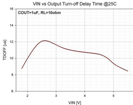
Fig. 16: Output Turn-Off Delay Time vs. Input Voltage
