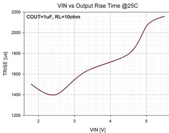
Fig. 19: Output Rise Time vs. Input Voltage
