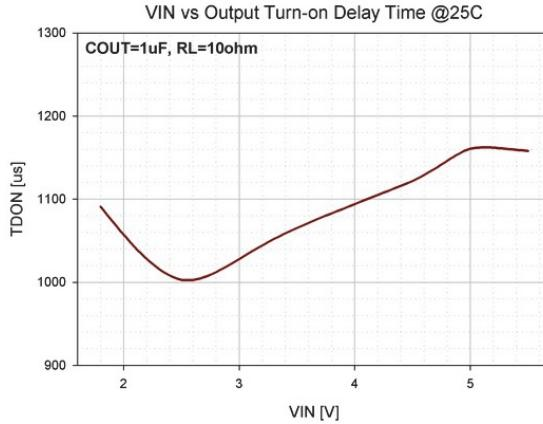
Fig. 17: Output Turn-On Delay Time vs. Input Voltage
