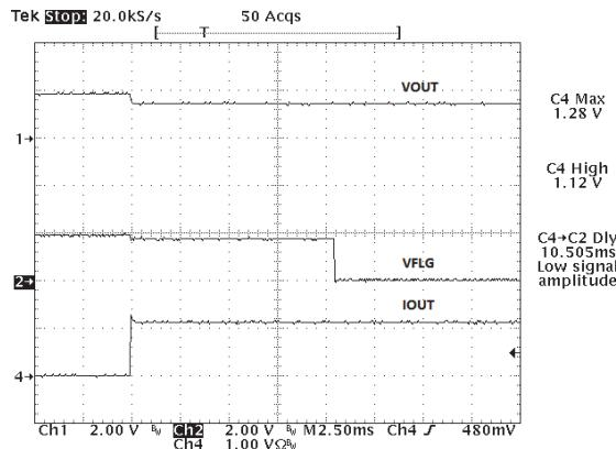
Fig. 27: Current Limit Operation (XRP2526-1):
