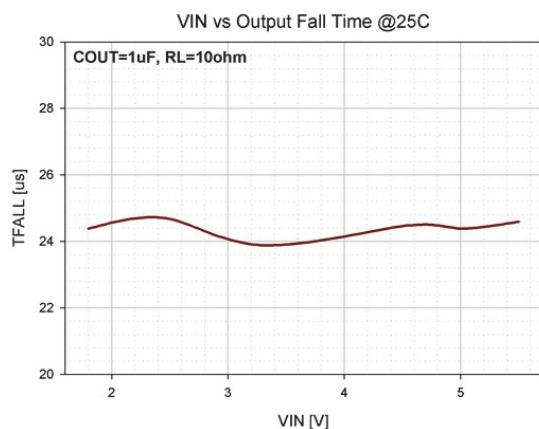
Fig. 18: Output Fall Time vs. Input Voltage
