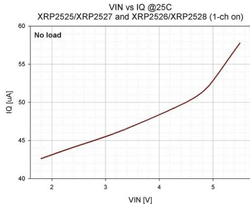
Fig. 10: Quiescent Current vs. Input Voltage
