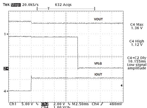
Fig. 26: Current Limit Operation (XRP2525-1):
