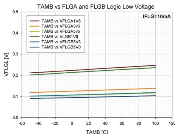
Fig. 9: FLG Logic Low Voltage vs. Temperature
