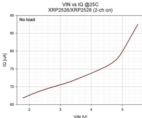
Fig. 11: Quiescent Current vs. Input Voltage
