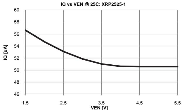
Fig. 23: Quiescent Current vs. Enable pin Voltage XRP2525-1
