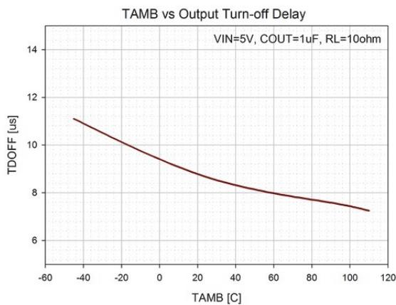
Fig. 12: Output Turn-off Delay vs. Temperature
