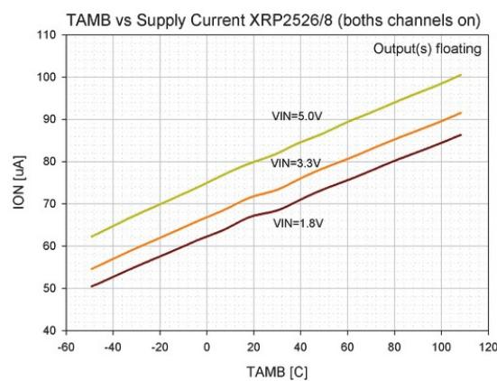
Fig. 8: Quiescent Current vs. Temperature XRP2526 (2-channels on)
