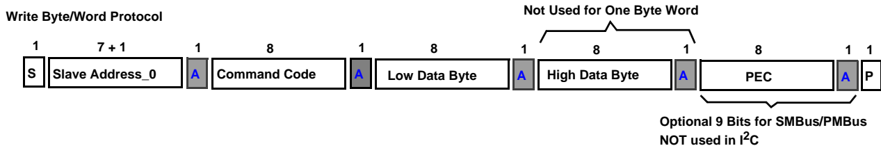
FIGURE 41. SIMPLIFIED SMBus/PMBus/I 2 C INITIALIZATION TIMING DIAGRAM WHEN BUS WRITE COMMAND SUCCESSFULLY RECEIVED
