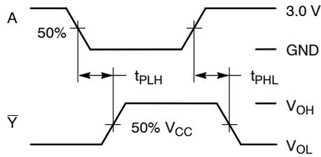
Figure 4. Switching Waveforms
