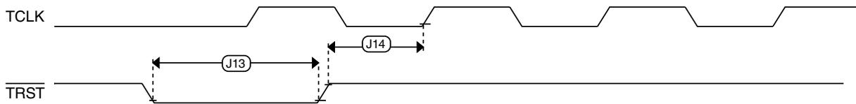
**Figure 10.  $\overline{\text{TRST}}$  timing**
