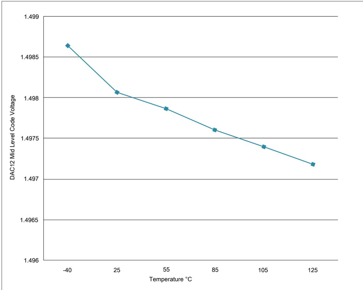
Figure 25. Offset at half scale vs. temperature
