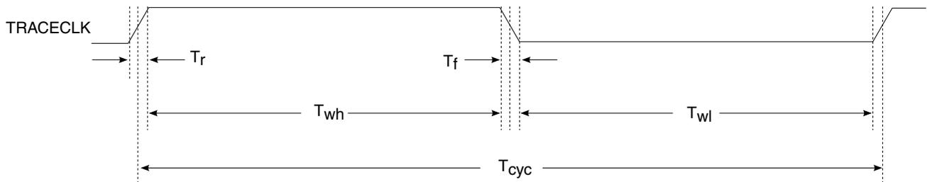
Figure 5. TRACE\_CLKOUT specifications
