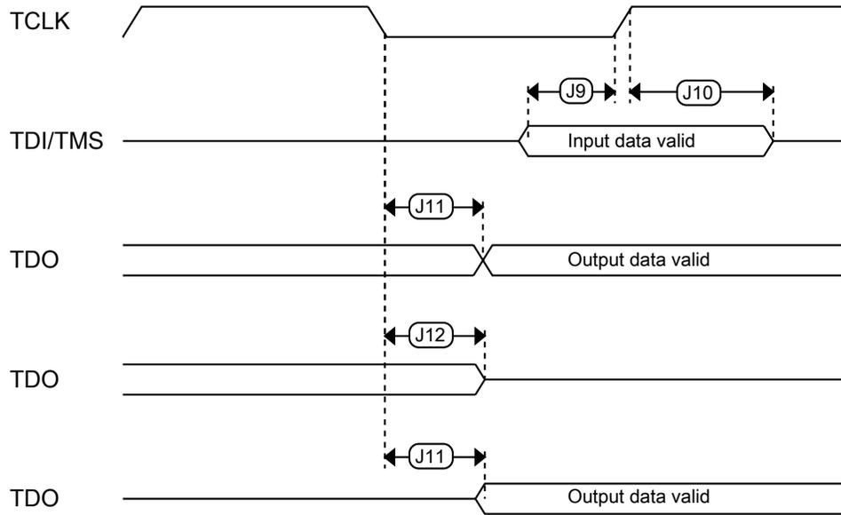
**Figure 9. Test Access Port timing**
