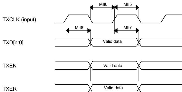
**Figure 26. RMI/MII transmit signal timing diagram**
