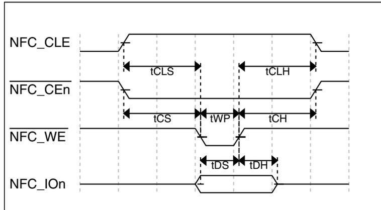
**Figure 12. Command latch cycle timing**
