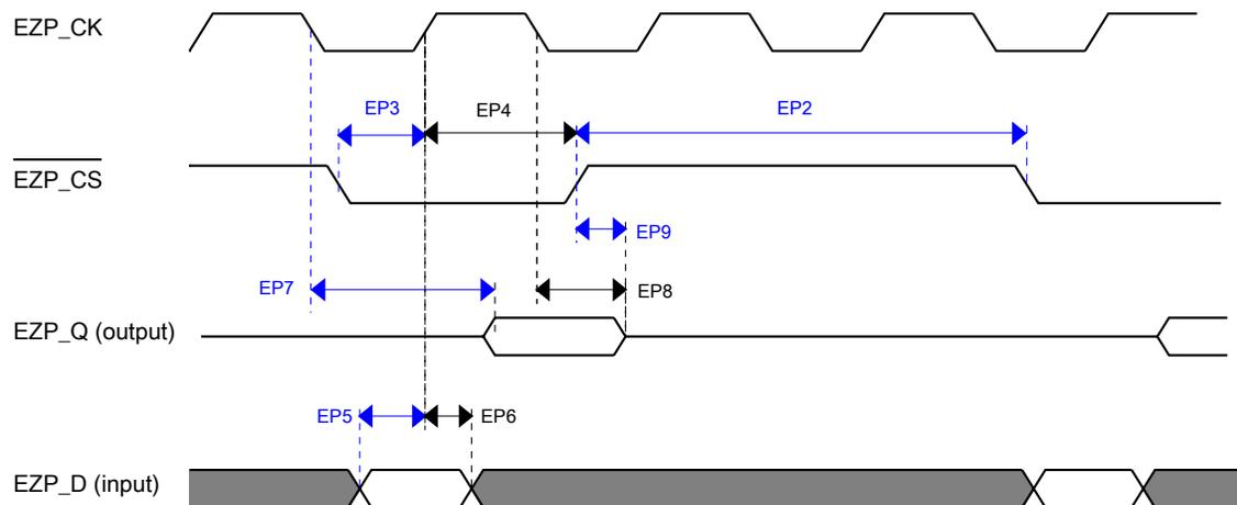
**Figure 11. EzPort Timing Diagram**
