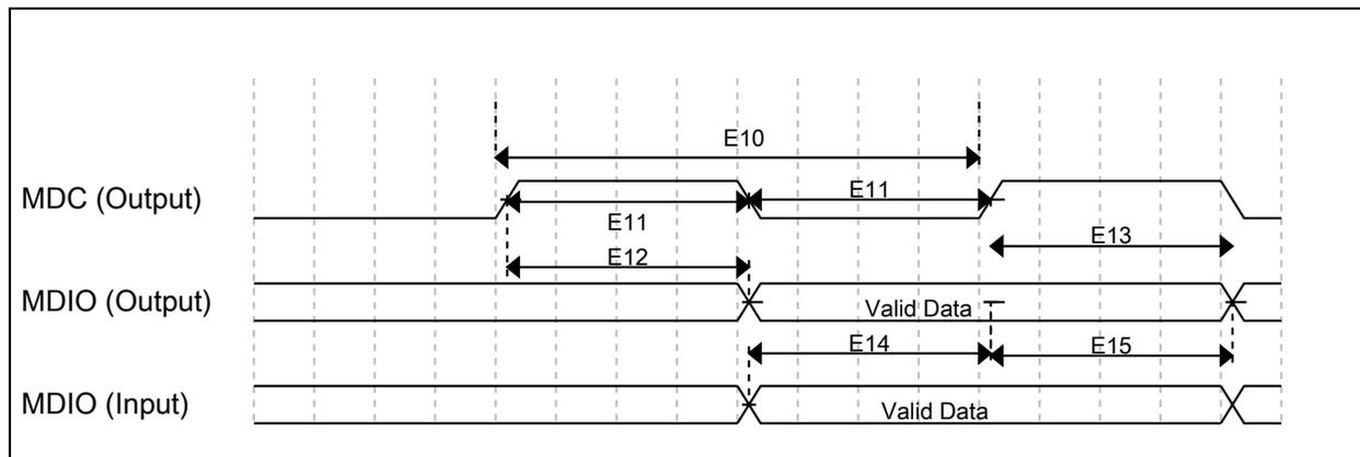
**Figure 28. MDIO serial management channel timing diagram**
