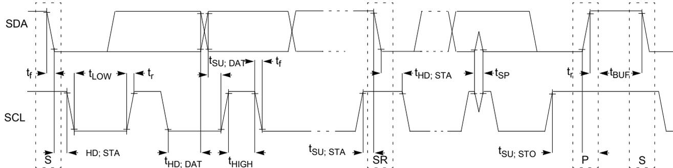
**Figure 33. Timing definition for fast and standard mode devices on the I<sup>2</sup>C bus**
