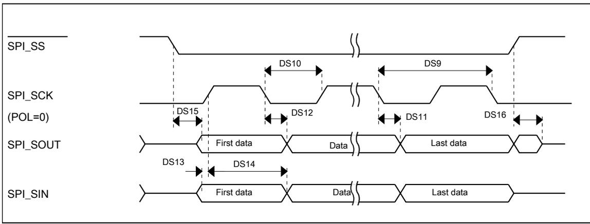
**Figure 30. DSPI classic DSPI timing — slave mode**
