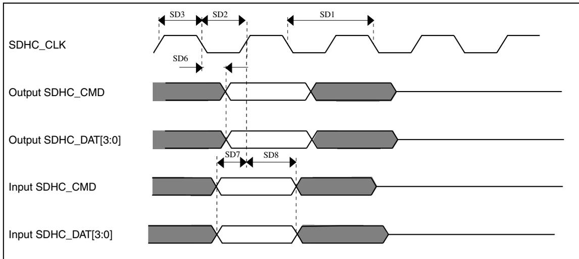
**Figure 34. SDHC timing**
