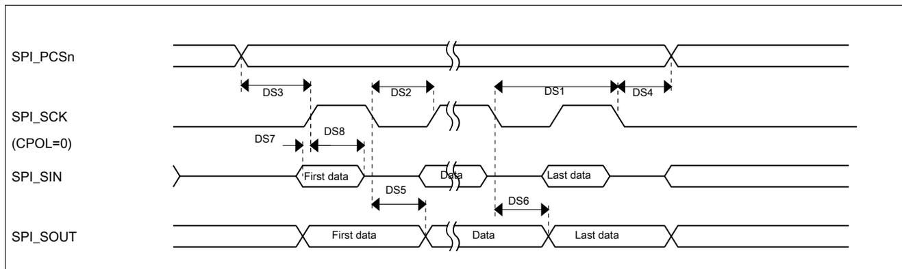
**Figure 29. DSPI classic DSPI timing — master mode**
