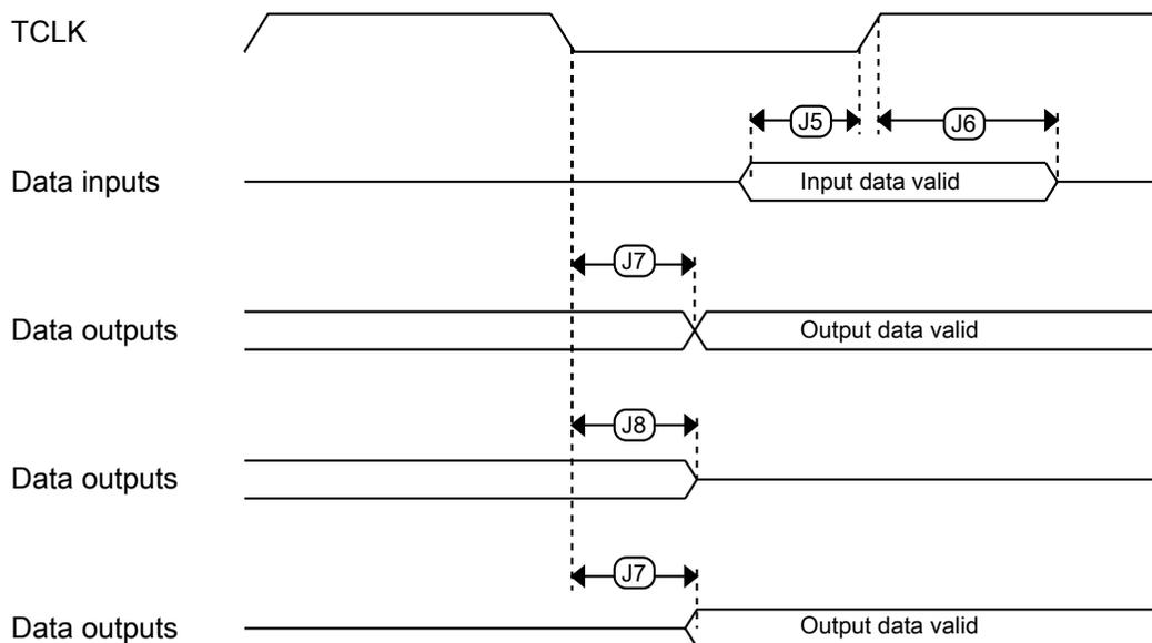
**Figure 8. Boundary scan (JTAG) timing**
