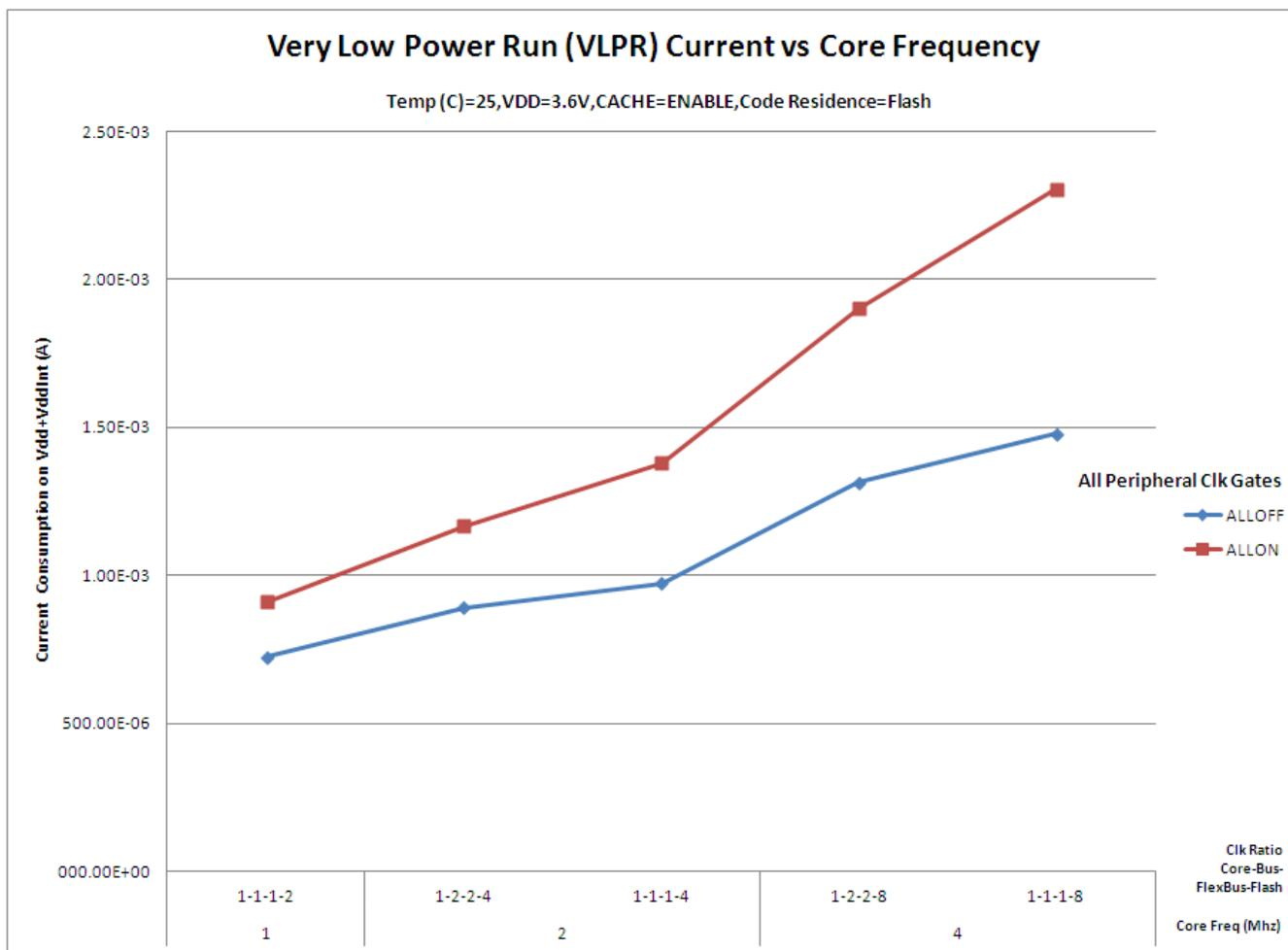
Figure 4. VLPR mode supply current vs. core frequency
