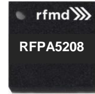
Package: Laminate, 10-pin, 4mm x 4mm x 1.05mm max
