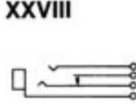
Single open (tip) circuit and single closed (ring) circuit. (J9).
