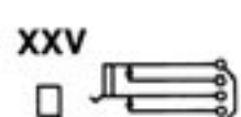
Single closed circuit. Isolated switching "break" circuit. Sleeve common to isolated switching circuit throw. (J4-1B).
