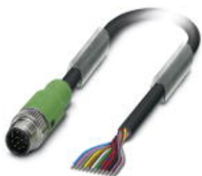
Sensor/actuator cable, 12-position, PVC, black RAL 9005, Plug straight M12 SPEEDCON, A-coded, on free cable end, cable length: 20 m
