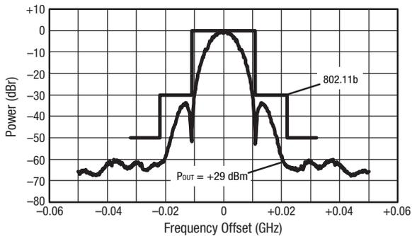
**Figure 7. Spectral Mask (11 Mbps, V<sub>CC</sub> = 3.3 V)**
