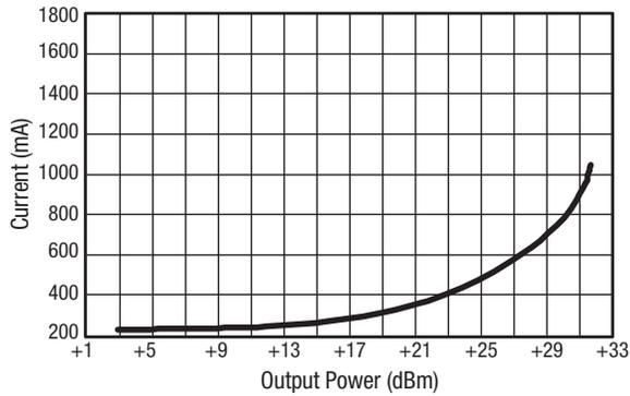
**Figure 5. Current vs Output Power (CW, V<sub>CC</sub> = 3.3 V)**
