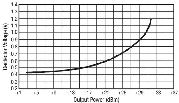
**Figure 11. Detector Voltage vs Output Power
