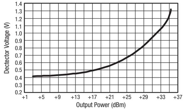
**Figure 10. Detector Voltage vs Output Power
