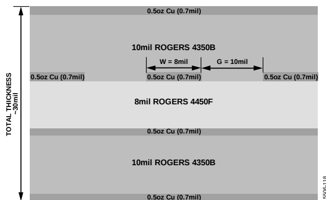
Figure 19. Evaluation Board Cross Sectional View
