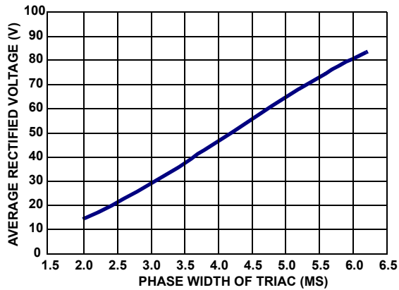
FIGURE 5. AVERAGE VOLTAGE vs ANGLE OF A TRIAC DIMMER
