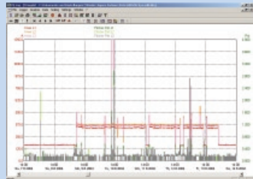
For root cause analysis, different measurements such as flicker, voltage and THD can be shown in the same time plot, helping to quickly identify the cause of a disturbance.
