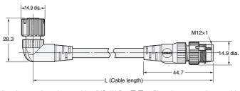
Note: Oil-resistant polyurethane cables (XS5W-D42 $\square$ - $\square$ 81-P) and spatter-resistant cables (XS5W-D421- $\square$ 81-SA) have black covers. Fire-retardant, robot cables (XS5W-D42 $\square$ - $\square$ 81-F), oil-resistant (polyurethane) robot cables (XS5W-D42B- $\square$ 81-PR) have warm gray covers.
