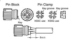
• Tentatively insert the pins to the pin block holes so that the key on the pin block will coincide with the key groove on the pin clamp. Then insert the cable along with the pin clamp.
