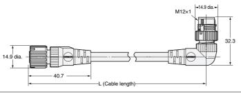
Right-angle (Socket)/straight (Plug) Fire-retardant, Robot Cable XS5W-D424-□81-F
