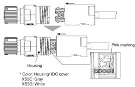
Note: Confirm that the color of the housing and the IDC cover is same before insertion
