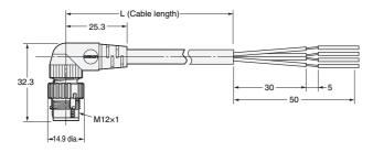
Note: Oil-resistant polyurethane cables (XS5H-D42 $\square$ - $\square$ 80-P) and spatter-resistant cables (XS5H-D421- $\square$ 80-SA) have black covers. Fire-retardant, robot cables (XS5H-D42 $\square$ - $\square$ 80-F) have warm gray covers.
