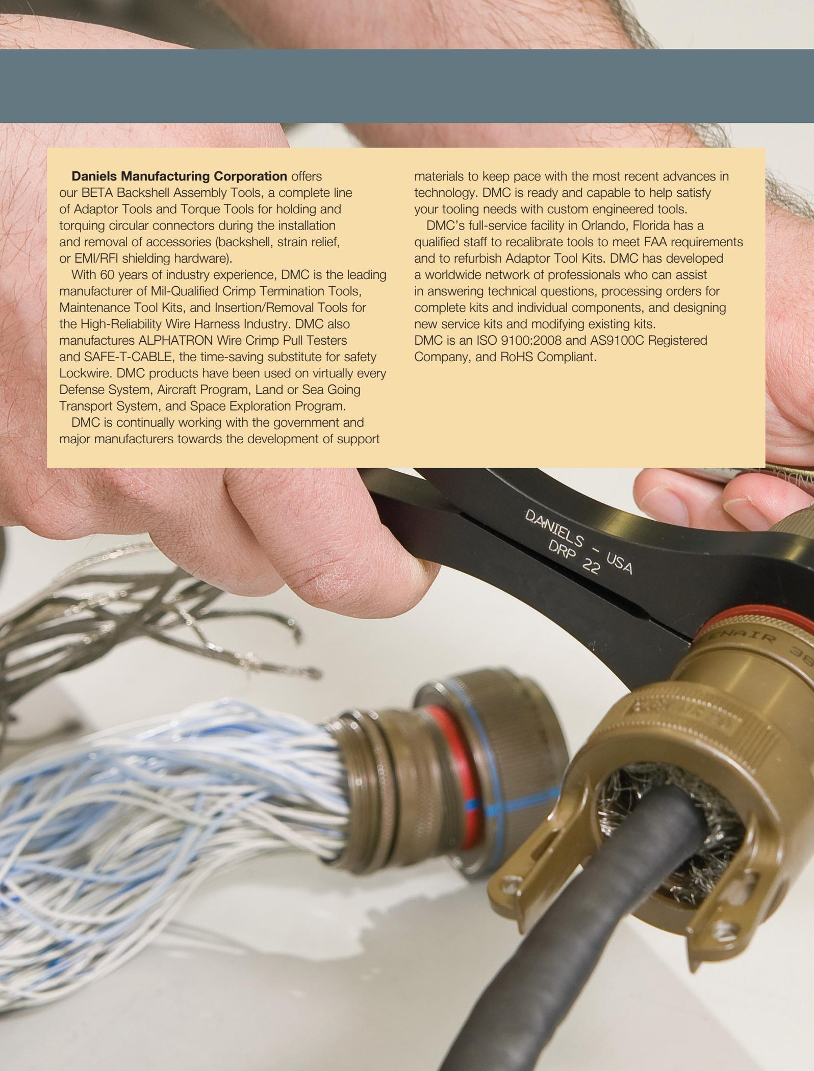
**Daniels Manufacturing Corporation** offers our BETA Backshell Assembly Tools, a complete line of Adaptor Tools and Torque Tools for holding and torquing circular connectors during the installation and removal of accessories (backshell, strain relief, or EMI/RFI shielding hardware).
