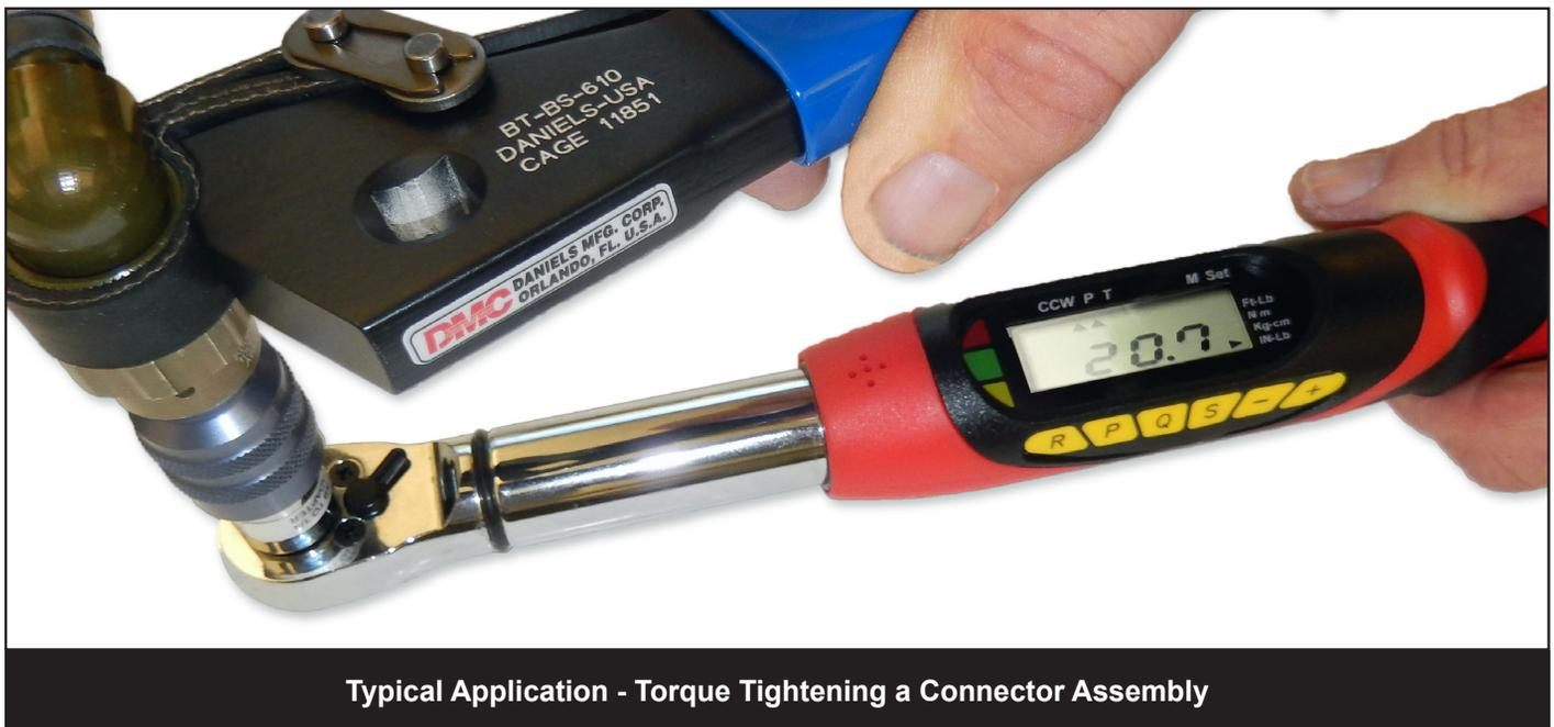
Typical Application - Torque Tightening a Connector Assembly
