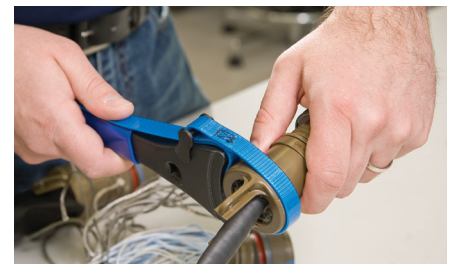
Strap wrench, strain relief, connector
