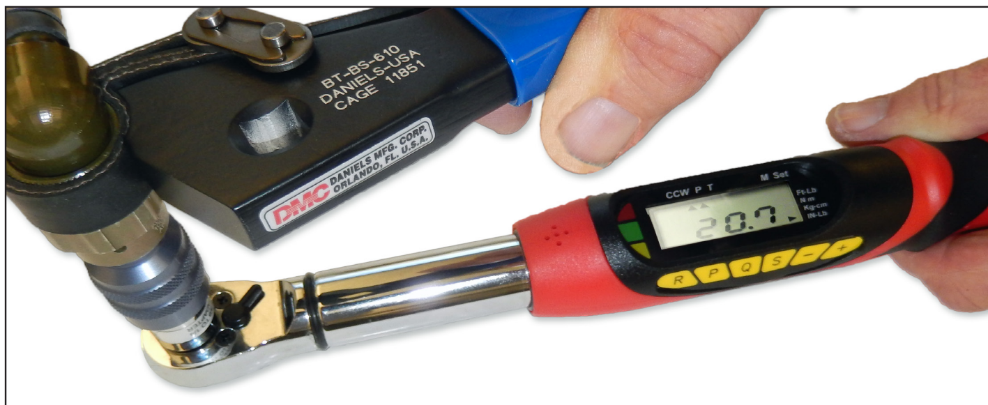
Typical Application - Torque Tightening a Connector Assembly
