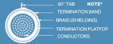
The 90° tab is then curled and folded back over the buckle using the rollover tool (applies to two-step only).
