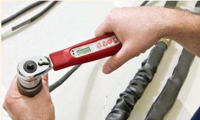
*Digital torque wrench, adaptor, connector, strain relief*
