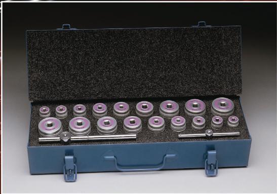
**The Adaptor Tool** - A vastly improved low cost assembly tool and system that solves existing problems in the assembly and maintenance of circular connectors and their rear accessories (Backshells). The Adaptor Tool works on a revolutionary principle; the socket like tool exerts pressure equally on the connector's keys and keyways preventing damage, distortion and false torque readings.
