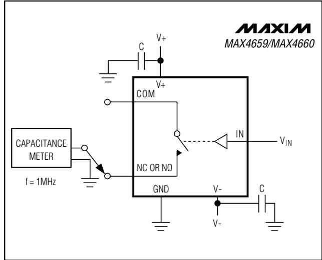
Figure 7. Channel Off-Capacitance
