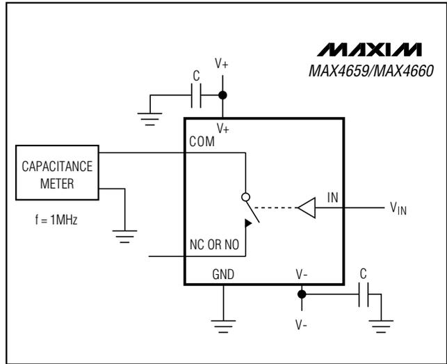
Figure 8. Channel On-Capacitance
