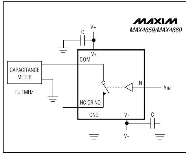
Figure 8. Channel On-Capacitance
