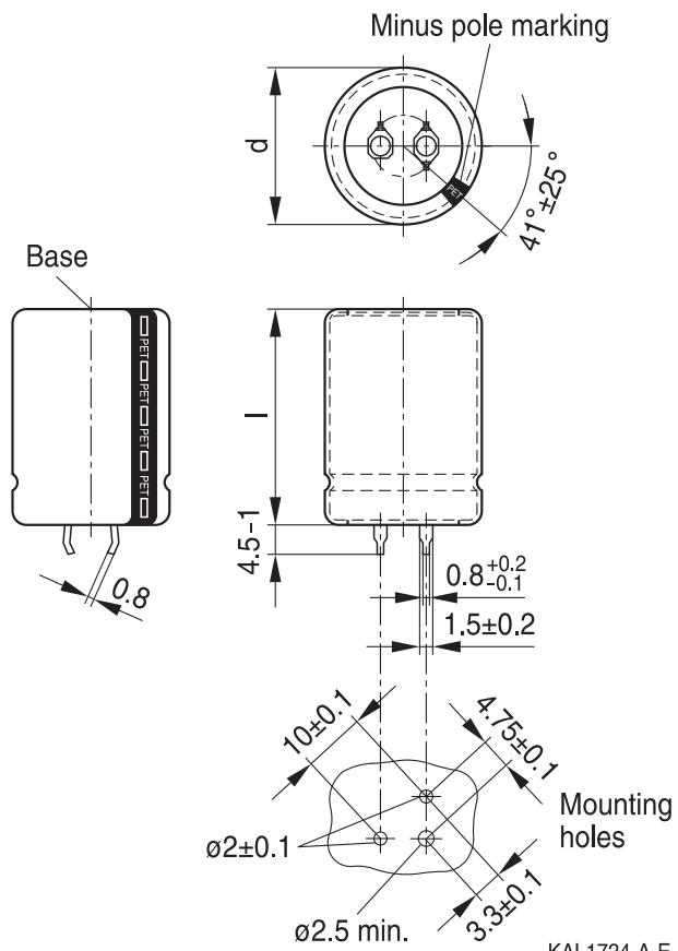
Snap-in capacitors are also available with 3 terminals (length (4.5 – 1) mm).
